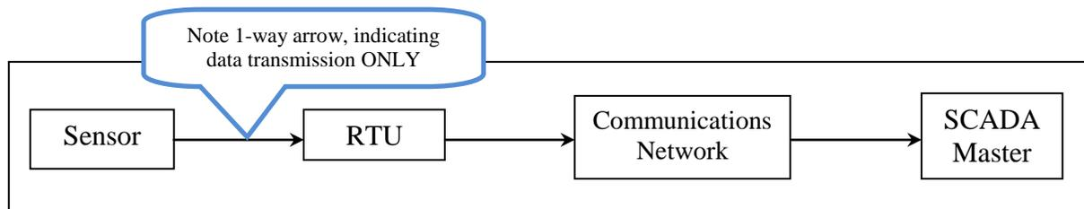
**Simplified Illustration of RTU Function in a SCADA System**
